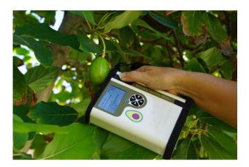
Based on the original F-750 Produce Quality Meter, is specifically engineered to gauge the maturity of avocados via dry-matter assessment. The instrument is designed to accurately predict percent dry matter straight out of the box with just a simple push of the button. Utilizing a wi-fi connection, the data collected using the F-751 Avocado Quality Meter can be seamlessly transferred to a computer for easy analysis and data sharing.
